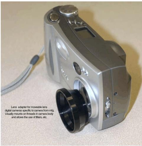
Lens adapter for moveable lens digital cameras specific to camera from mfg. Usually mounts on threads in camera body and allows the use of filters, etc.
