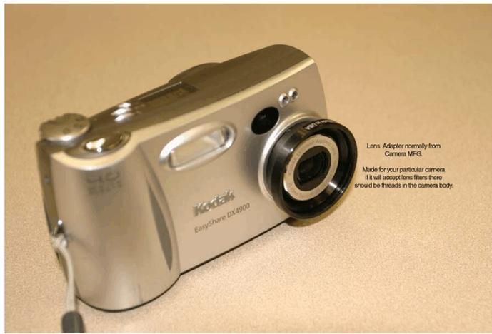
Lens Adapter normally from Camera MFG. Made for your particular camera if it will accept lens filters there should be threads in the camera body.
